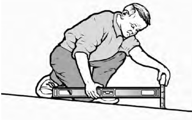
Measuring slope using a 24 inch bubble level and tape measure
